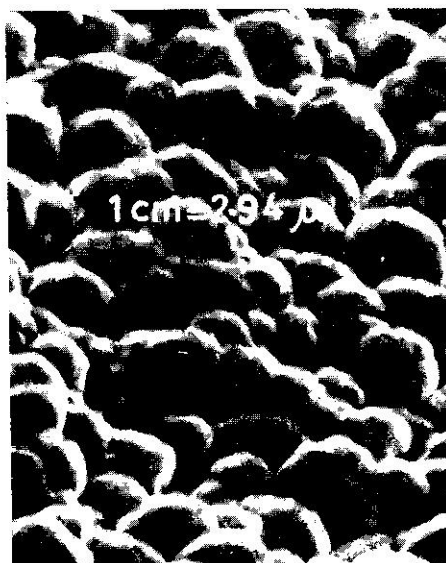
Fig. 3. Scanning electron micrograph of a deposited film of \text{PbO}_2 .
